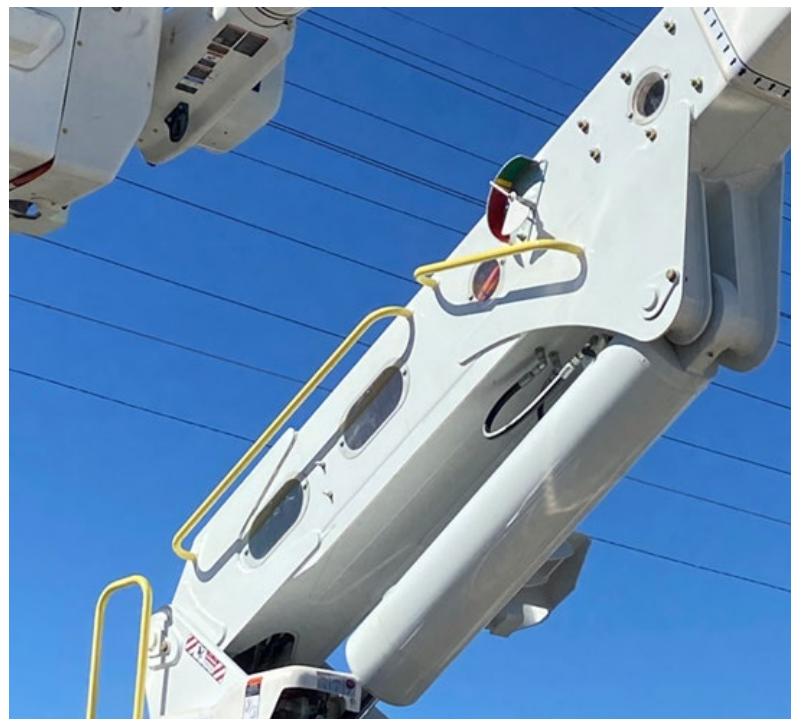
Figure 1: Angle Gauge Installed on Lower Boom
