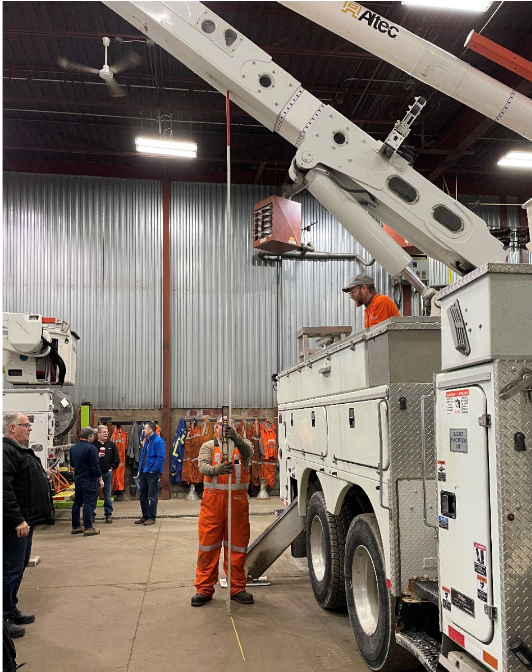
Figure 3: Boom Height Measurement
