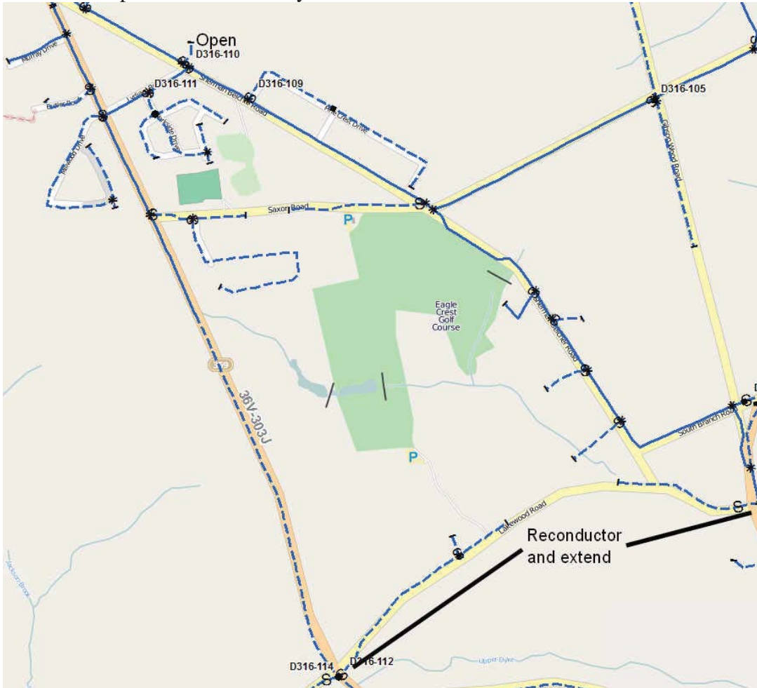
Figure 11 36V-303 Load Transfer Part2
