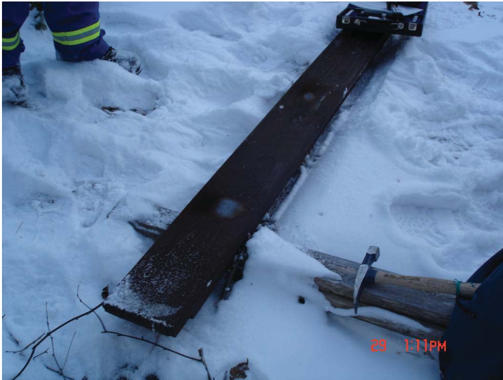
Photo 17 – Hardness Testing of Spare Roller Path Plate (32 mm)
