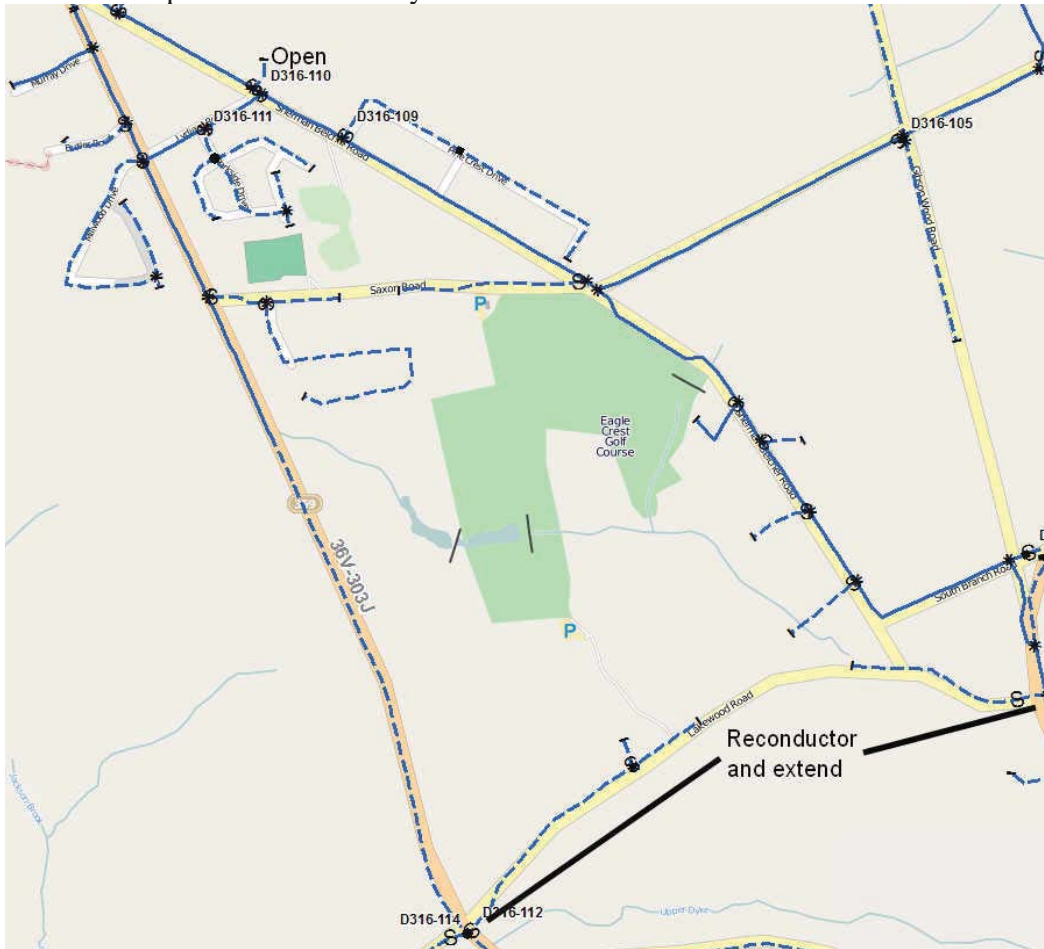
Figure 11 36V-303 Load Transfer Part2
