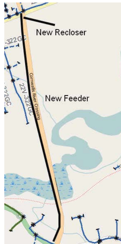
Figure 4 99V-3X4 New Feeder Construction Part-2
