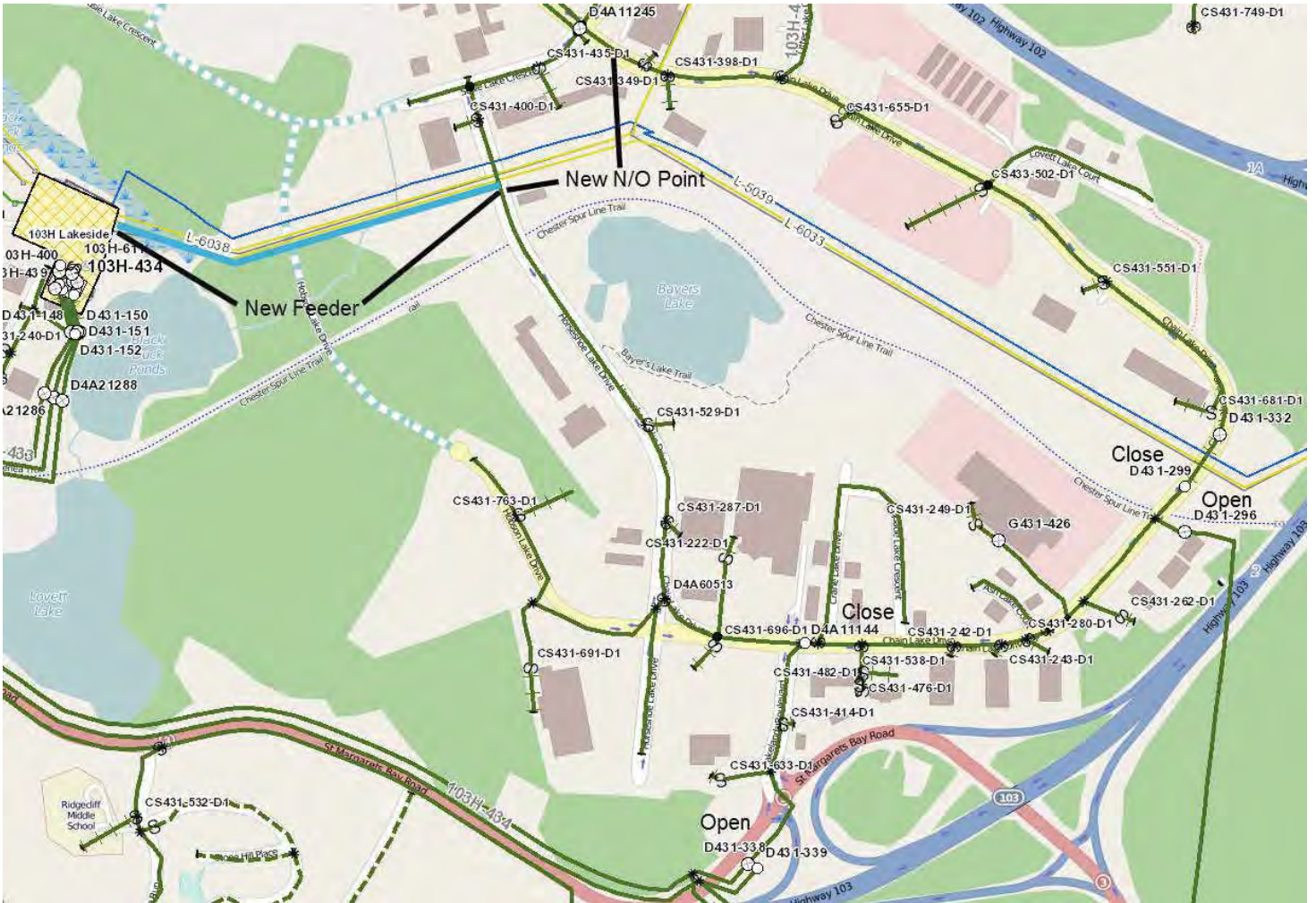
Figure 12 Alternative 103H/129H-A; New 103H-Lakeside Feeder
