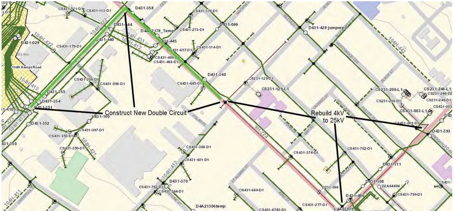
Figure 6 Alternative A; 104H-Kempt Road New Feeder-A
