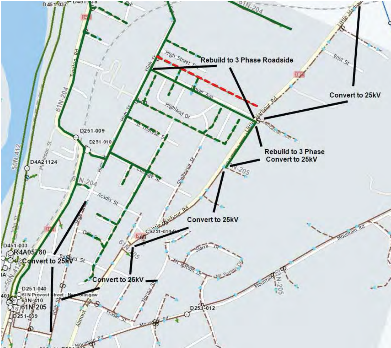
Figure 25 Little Harbour Road Conversion (61N-Provost Phase 3)
