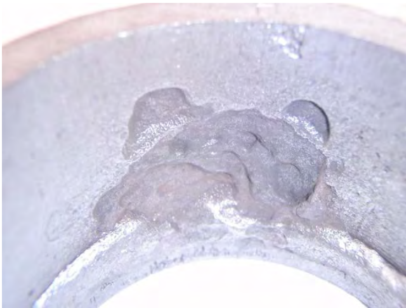
Photograph 27 Hot Side After Final Vibration of Deposit
