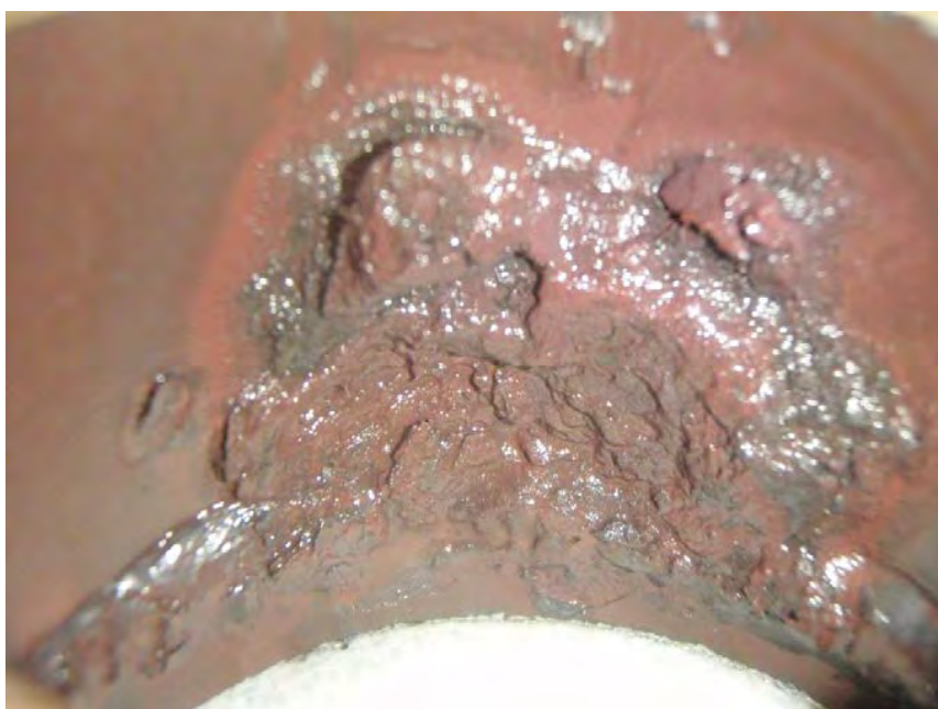
Photograph 5 Ammonium Bromate, 48 Hours, Hot Side (Water Rinsed Before Photograph)
