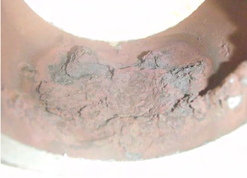
Photograph 13 Ammonium Bromate, 72 Hours, View from Bottom
