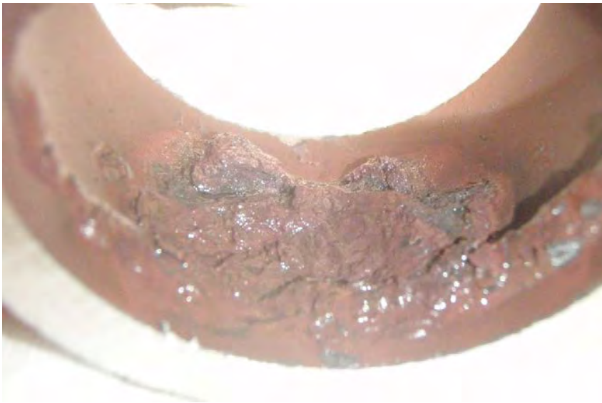
Photograph 7 Ammonium Bromate, 48 Hours, Hot Side, View from Below
