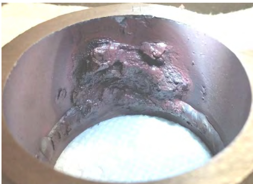
Photograph 4 Ammonium Bromate at 30 Hours, Hot Side – Right Side Exposing Iron Oxide
