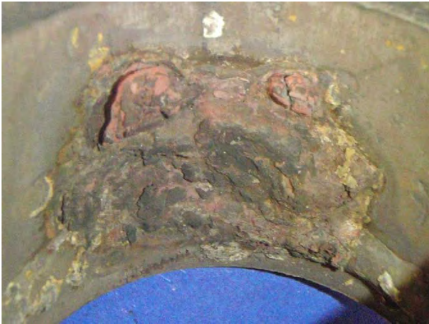
Photograph 15 End of 2 nd Stage (EDTA at 24 Hours), Iron Oxide Removal Stage, Hot Side Crown
