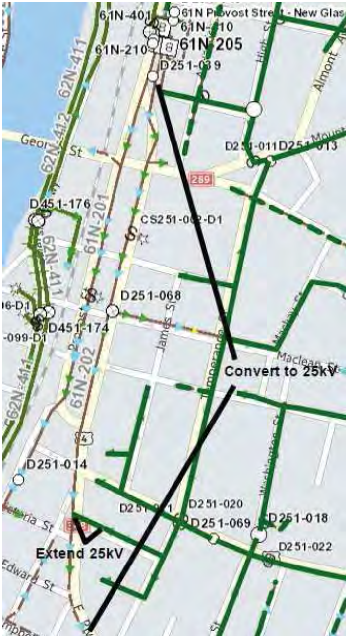
Figure 31 Archimedes Street Conversion (61N-Provost Phase 5)
