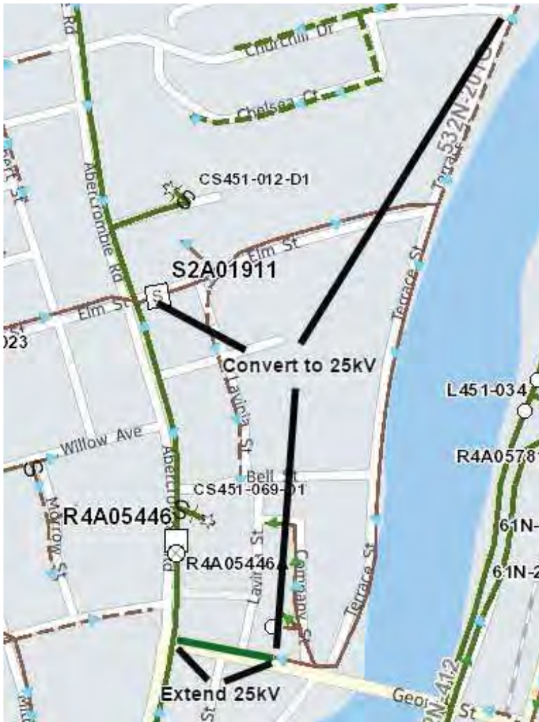
Figure 17 Terrace Street Conversion (532N-Elm Phase 1)
