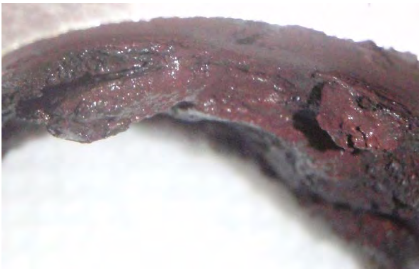
Photograph 10 Ammonium Bromate 56 Hours, Top View
