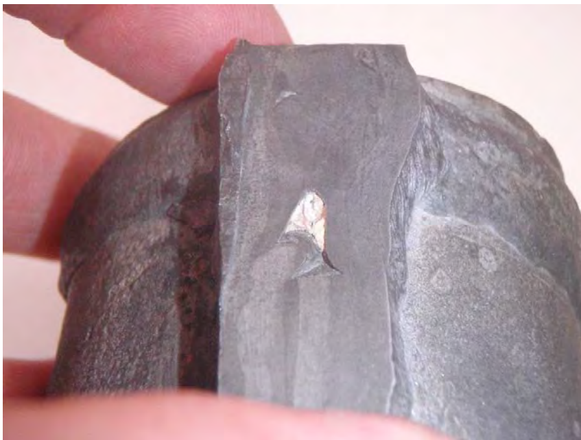
Photograph 26 Membrane After Bead Blast, Example of Flux Inclusion in Weld
