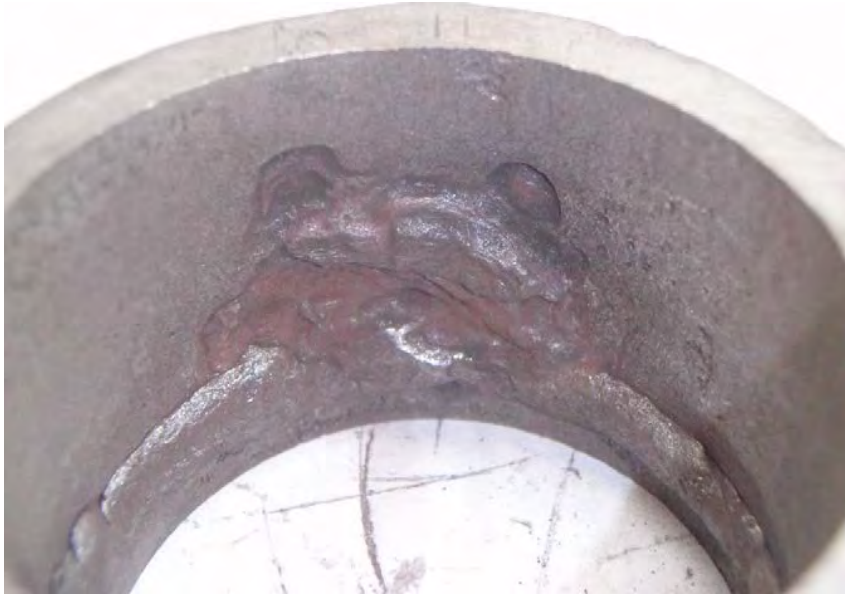
Photograph 23 Hot Side After An Hour of Vibration of Surfaces
