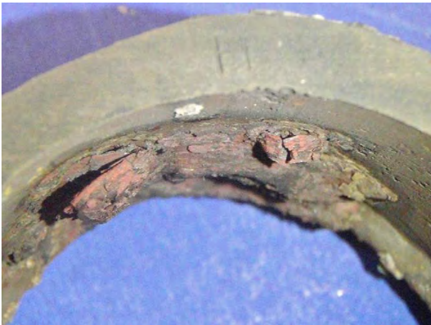
Photograph 16 End of 2 nd Stage (EDTA at 24 Hours), Iron Oxide Removal Stage, Hot Side Top View
