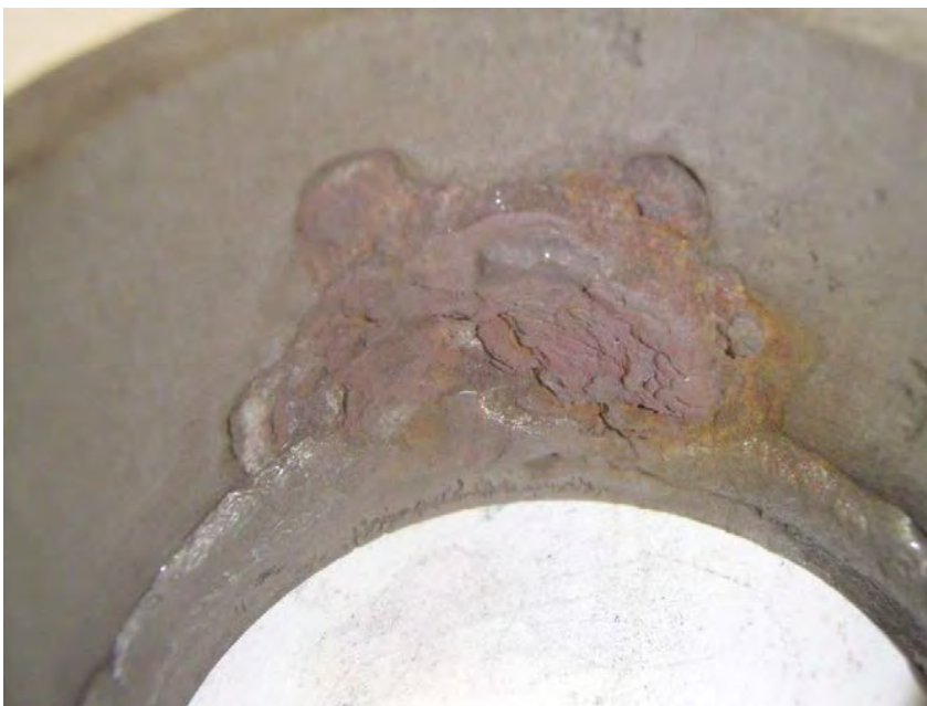
Photograph 22 Hot Side After Brushing and Scraping Brushing and vibrating removed 5.30 g/ft 2 and 6.23 g/ft 2 , respectively.
