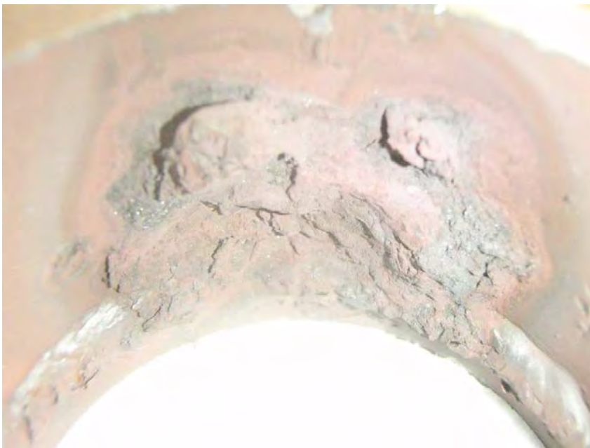
Photograph 11 Ammonium Bromate, 72 Hours Hot Side After Rinsing and Air Drying
