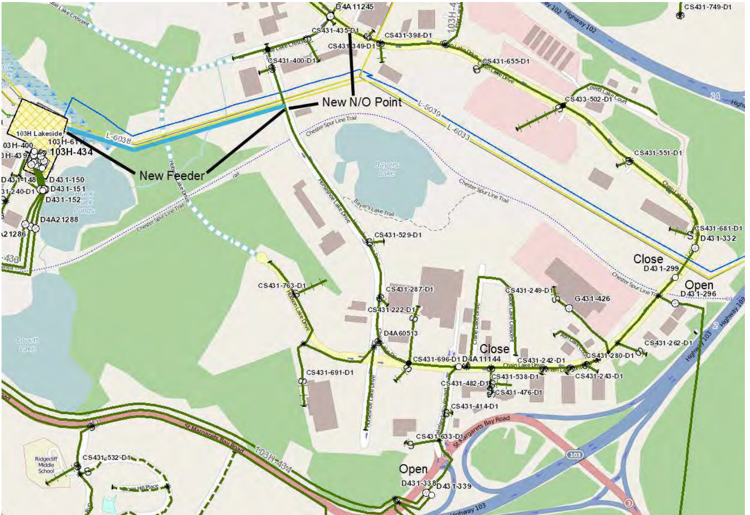
Figure 12 Alternative 103H/129H-A; New 103H-Lakeside Feeder
