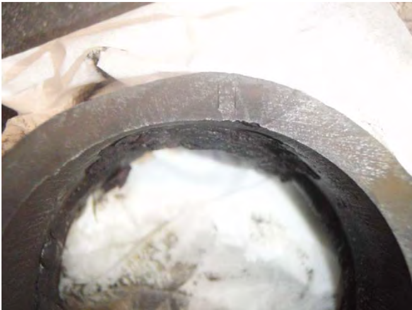
Photograph 20 Deposit Thickness at End
