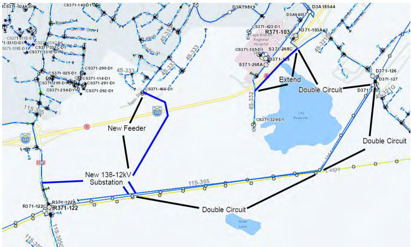
Figure 18 2016 New Prime Brook Substation
