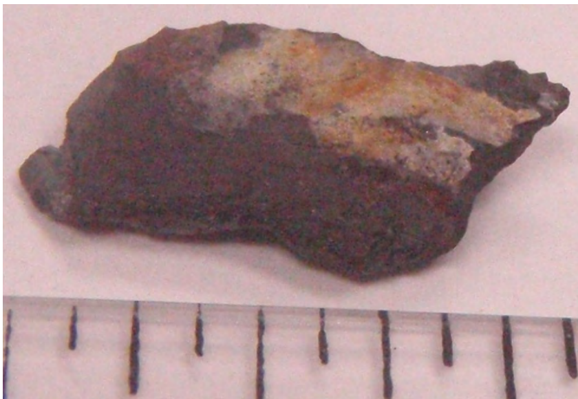
Photograph 28 Underside of 9/16 Inch Long Chunk That Was Removed Dur- ing Final Vibration (Top was dull gray color.)
