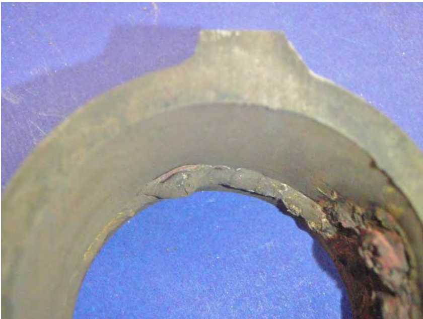
Photograph 14 End of 2 nd Stage (EDTA at 24 Hours), Iron Oxide Removal Stage, Membrane and Cold Side
