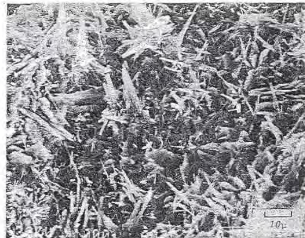
Fig. 11 Scanning electron microscope photograph of tricalcium sulphoaluminate crystals in an insulator cement at 1000 X.
