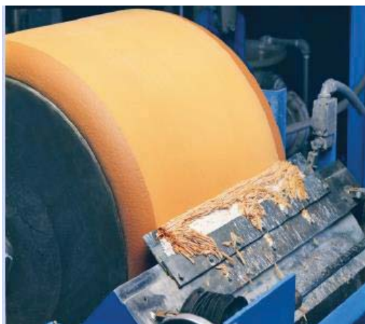
Figure 1: Dry cake being scraped off of a pre-coated filter drum (www.alarcorp.com)
