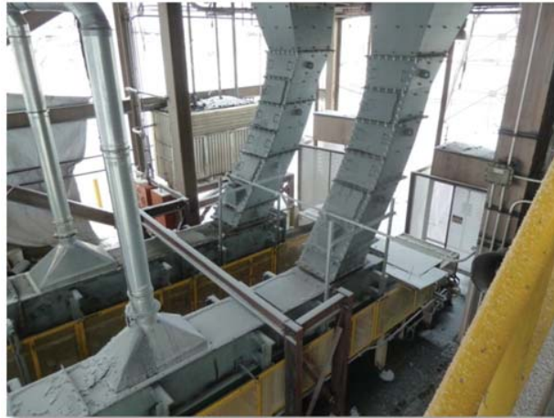
Example of Improved CDG Designed Chute and Loading Zone
