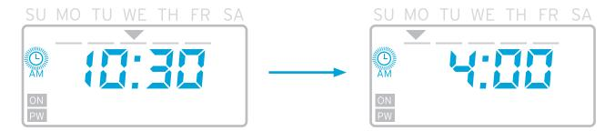
**3.** Press the **WRITE** Key. The colon on the display flash and the clock will start. Press the **MODE** Key 3 times to return to the run mode. Note: The set time is enabled when the **WRITE** Key is pressed.
