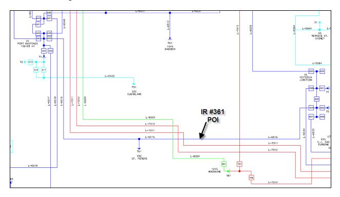
L-6516 is classified as a "NERC critical transmission element", and therefore generation connections to this line require a three-breaker ring bus.
