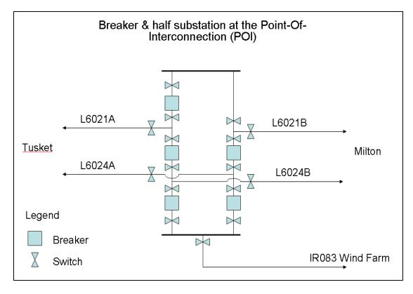
This substation configuration will offer the advantage of avoiding overloading L-6021B and L-6020 during system normal light load, thus avoiding the cost of
