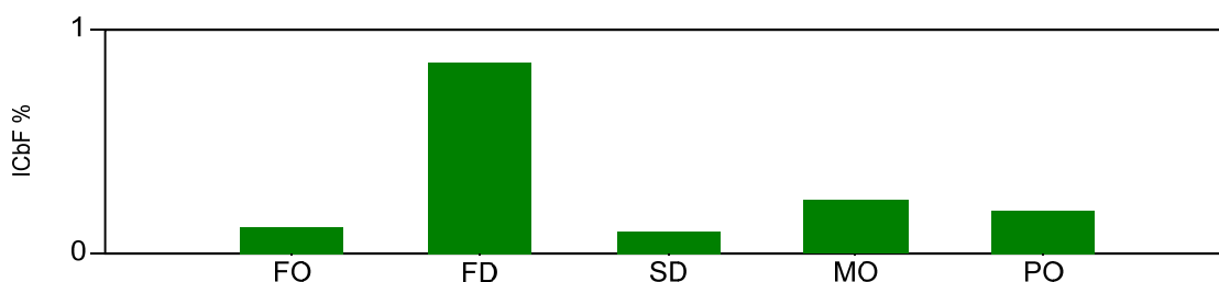
Plant Aux. Processes and Services ICBF by event type for Fossil units based on 2004-2008 data.
