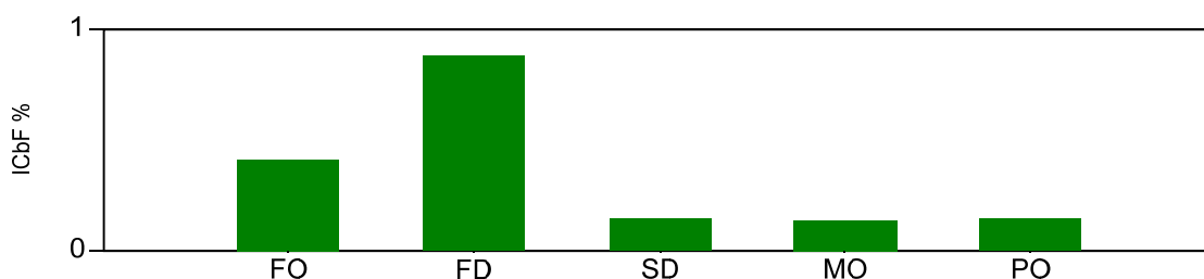
Instrumentation and Control ICBF by event type for Fossil units based on 2004-2008 data.
