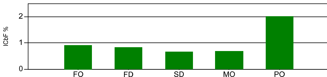
Steam Turbine ICBF by event type for Fossil units based on 2004-2008 data.
