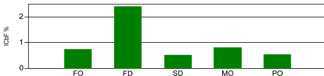
Heat Power Cycle ICbF by event type for Fossil units based on 2004-2008 data.
