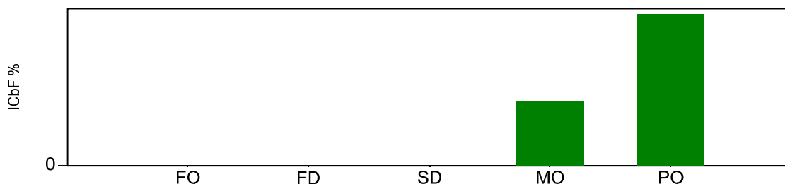
Buildings and Structures ICbF by event type for Fossil units based on 2004-2008 data.
