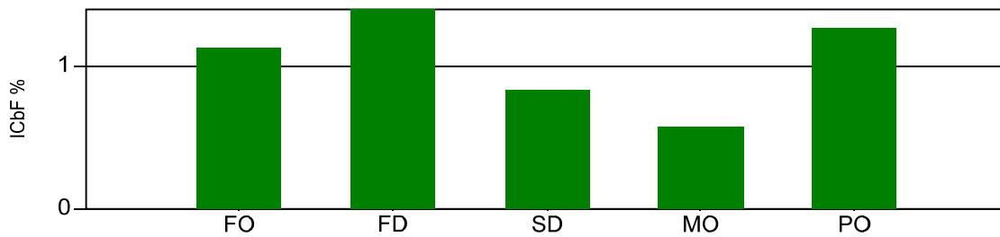
Steam Turbine ICBF by event type for Fossil units based on 2005-2009 data.
